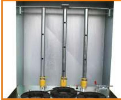
A powerful, automatically-operated reverse pulse cleaning system is built into the underside of the weatherproof lid.
